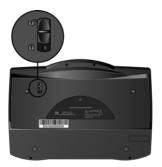
**Note:** The locking tab protects the scanner's scan head by holding it securely in position. Lock the scanner when transporting it from one location to another, but remember to unlock it before scanning. The scanner will not scan when locked.
